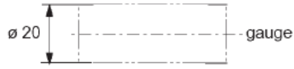
Fig. 9.7 Gauge boundary for GD&T according to Fig. 9.6
